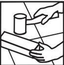
Level the surface with the help of a wooden jig and rubber mallet.
