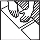
Proceed regularly by placing joint surplus between the tiles.
